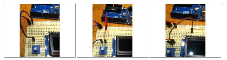
• Now we will hook up the contrast pot. Connect one side of the pot to GND and the other to 5V. Then hook the middle of the pot to pin 3 on the display.
